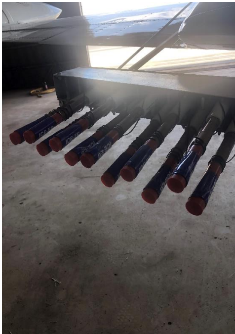
Left wing with glaciogenic flares. These flares are 75 gr AgI hygroscopic flares.
