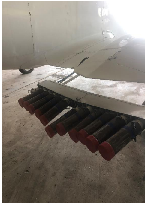
Right wing with hygroscopic flares These flares have 1/2 kilo (approx. 1.1 lbs.) of CaCl.
